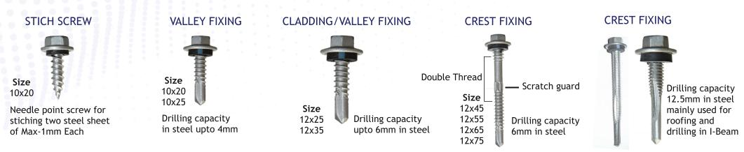
SPECIAL FEATURE: Additional Teflon Coating is provided to resist abrasion on screw during drilling and tapping
